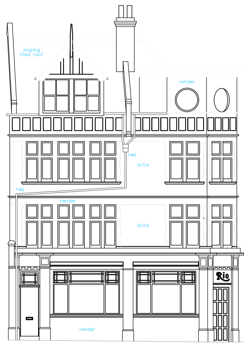
4 Existing Front Elevation Scale: 1:100
